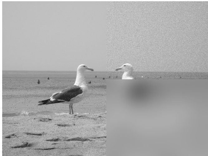
Figure 3: Gaussian noise, Gaussian blur and salt-and-pepper noise with an equal MSE of 275. The original is displayed in the upper left quadrant. 3
